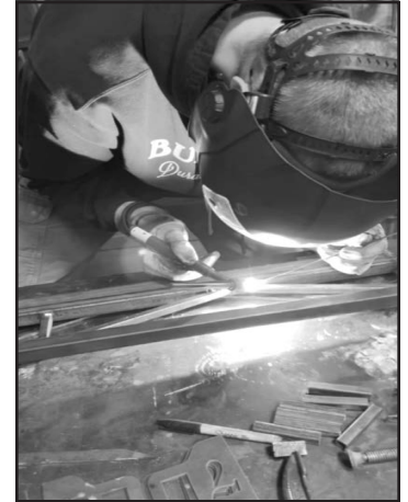
Steel Bridge team member, Kash Landry, welds a joint on a stringer for this year's bridge
