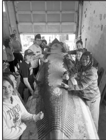
The concrete canoe team begins to apply another layer to this year's canoe "Peaches and Magnolias"
